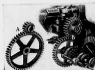
Gears for obtaining four different cutting lengths: \frac{1}{4} in., \frac{1}{2} in., \frac{3}{4} in. and 1\frac{1}{2} in.
