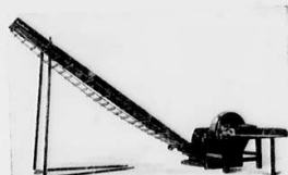
Carrier may be set to deliver to the right or left of the cutter.
